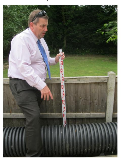
**Photo 8** shows the 2017 close in measurement of the land in the south western corner of No 49. The horizontal batten on the fence panel is the 3rd batten from the top of the fence (i.e. the batten nearest the ground). This shows the land raising is around 800mm in this area as the land is below the other piece of wood in the picture.
